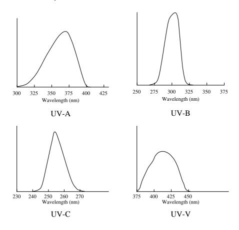
Figure 24. Spectral Response Curves.
