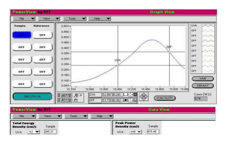
Figure 21. Cursor Measurement (Cursors on either side of a peak)
