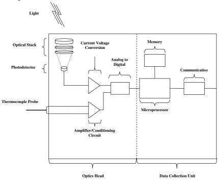
Figure 3. UV PowerMAP and UV MAP Plus block diagram.
