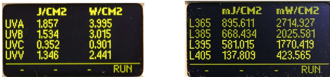
Figure 1: Display screens from broadband (left) and LED (right) multichannel radiometers
