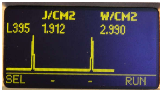
Figure 6: Irradiance and Energy Density values-single band instrument, dual LED
