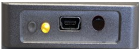
Flashing Yellow LED: Unit in Pause
