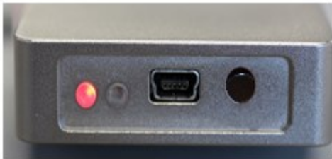
Flashing Red LED: Unit On and in Standby mode
