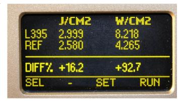
**TOGGLE** Mode– Pressing the **SEL** button, the user can "toggle" between the **GRAPH** mode and **REFERENCE** mode. TOGGLE Mode is only available on single band instruments
