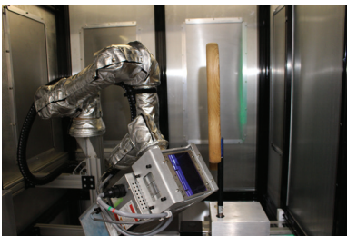
Figure 6. Flexibility of the robotic arm moving the UV source over guitar body for uniform curing. Image courtesy EIT LLC.
