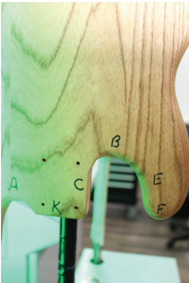
Figure 5. Guitar body with different test areas (letters) marked to allow for testing the exposure and cure conditions. Image courtesy EIT LLC.
