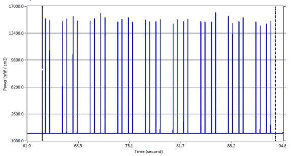
The graphic above shows 34 individual LED peaks collected over 30 second interval at a speed of 400 fpm at a sample rate of 2130.5 Hz. The consistency between the left and right LED in the above example is good.
