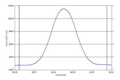
PowerView III allows the user to zoom in on a single LED pass. The time between the cursors is 0.03 seconds. At a sample rate of 2130.5 Hz, this equates to 64 individual sample points on the irradiance profile.
