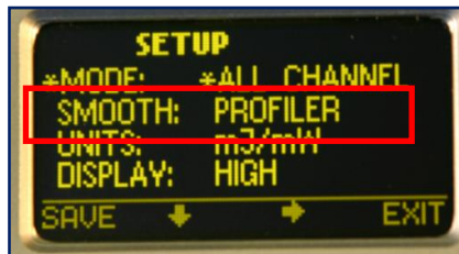
Right: Display referring to SMOOTH PROFILER (Sample Rate)
