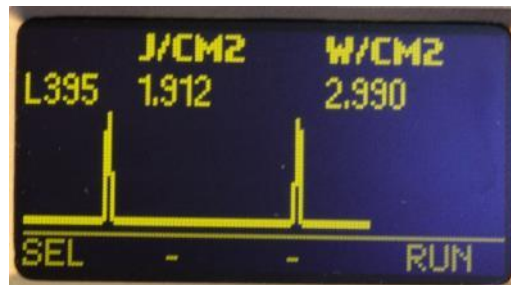
Figure 16: Display from LEDCure that shows the collected values and that the instrument passed under two arrays
