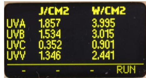
Figure One: Display showing Energy Density and Irradiance values in four bands
