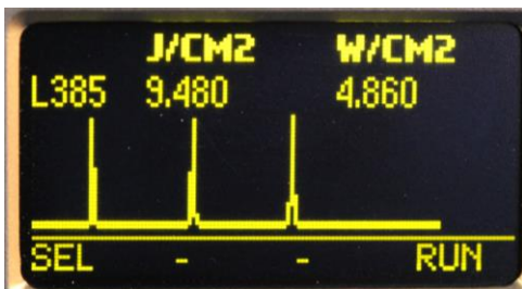
Figure Three: Exposure to three sources with similar intensity values
