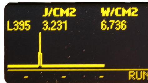
Figure One: Display showing Energy Density and Irradiance values in four bands
