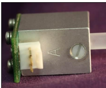
Figure 41 (Above Left): Close up showing the set screw holding the Quartz Rod in place.
