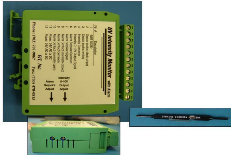
Figure 28: DIN Rail UV Intensity Monitor Alarm and Intensity Adjust Potentiometers
