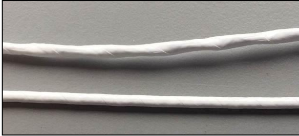
Figure 29 Top: Twisted (T-Type) three-wire cable used with the EMI Compact Sensor
