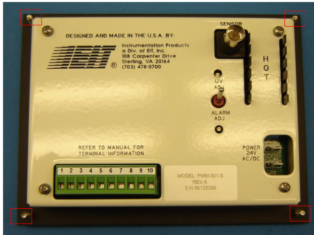
Appendix E Figure 4: Online UV Intensity Display Module Mounting Studs
