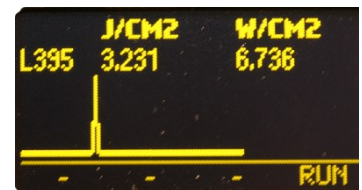
Top: LEDCure Radiometer Above: LEDCure Display Screen Far Left: L395 Total Measured Optic Response Left: Profiler Comparison of LED at different heights from the substrate
