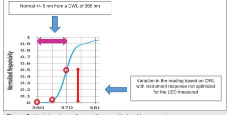
Figure 3. Variation in readings with nonoptimized instrument
