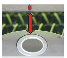
Figure 1. Index marks to align optics.
