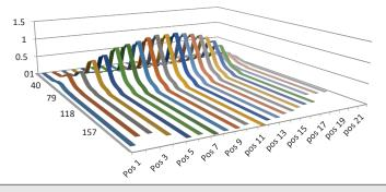
**Figure 2.** Uniformity of an arc lamp in 21 different positions across the width and length of the bulb. Courtesy of Jenton International Ltd. (UK)
