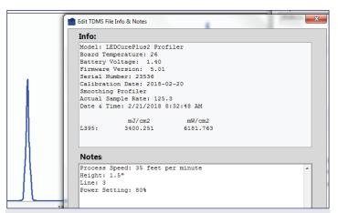
**Figure 3.** This data collection and analysis software allows operators to record notes about the system that become integrated with the data.
