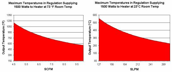
\*Note: Red area is achievable temperatures at various flow rates. Maximum values on graph will be less at lower ambient temperatures and/or lower available heater power. Maximum flow rate will decrease as temperature goes up.
