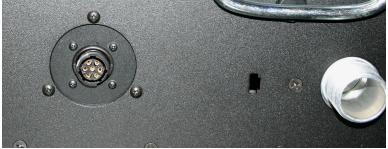
**Figure 4**-(Above) Heater Power/Sensing connection on left, hose connection on right **Figure 5**-(Below) Heater Power/Sensing cable and Heater Hose shown connected
